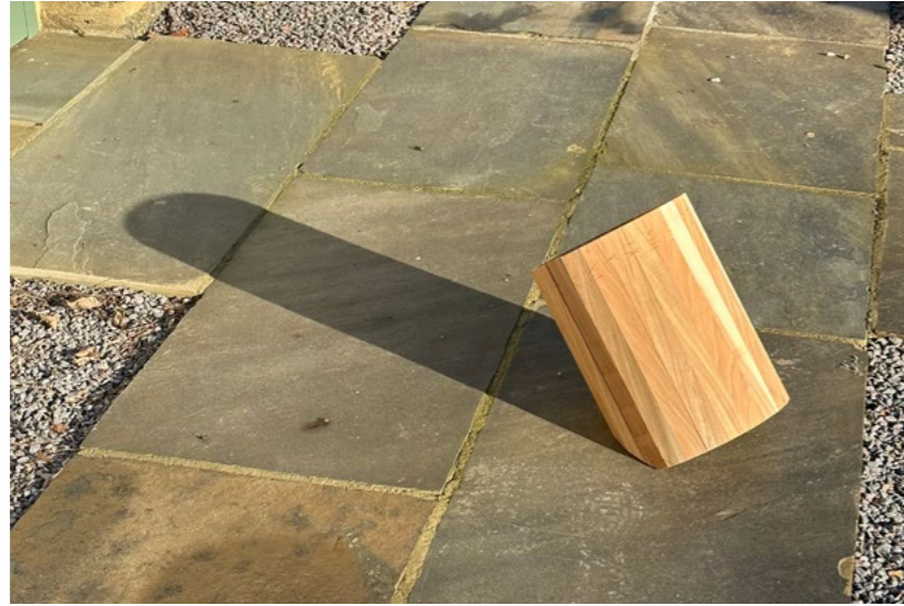
A hollow prototype made from 24 panels of western red cedar proved the sundial concept.
