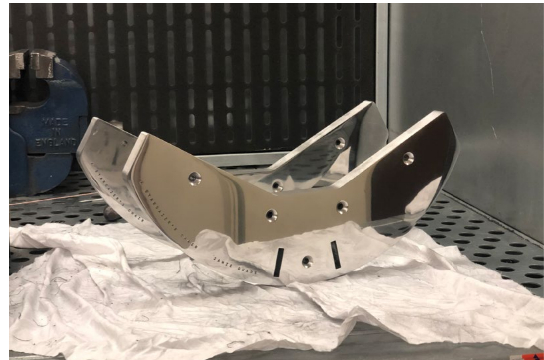
20mm thick altitude bearings were engraved, then polished by hand to a high shine.
