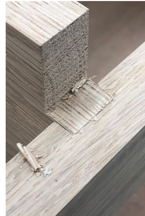
While designed predominantly for machinery processes, final touches were achieved using chisels.
