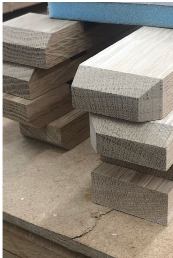
Heavily chamfered feet help guide the table top onto the base.
