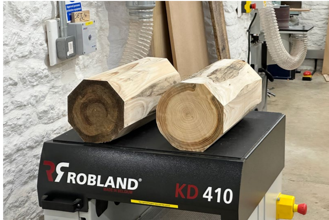
Four more faces were cut using a jig to cradle each log at 45°, resulting in an octagonal shape. These eight faces were marked for later steps.
