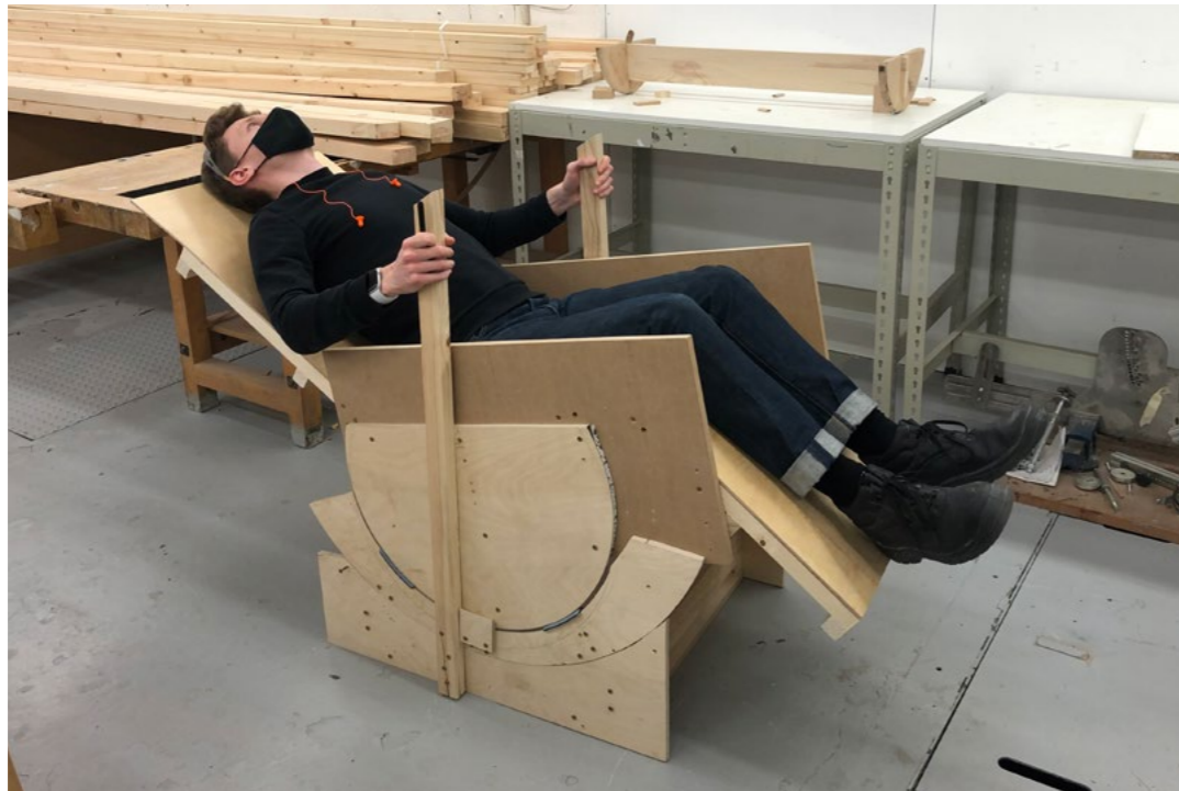
The reclining method was developed from the Dobsonian telescope; using PTFE pads running against a large semicircular edge.
