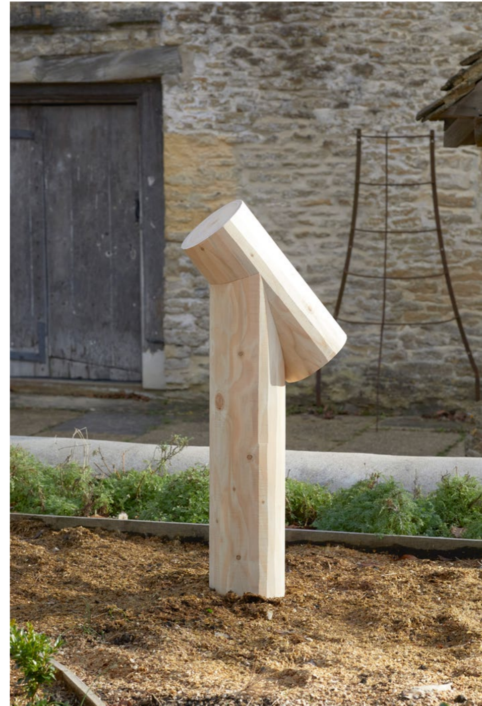
② Western red cedar's outdoor durability and lightness makes it a desirable timber for use as a sundial.
