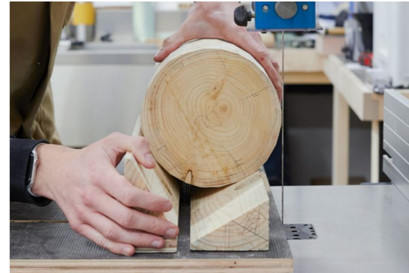
② A 30° cradle allowed for eight more faces to be cut. The piece was then flipped and the process repeated to total 24 faces.
