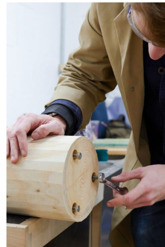
② Three adjustable feet were installed to enable level footing on uneven ground.
