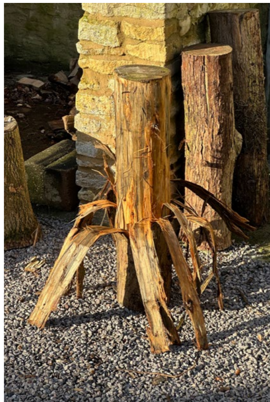
The logs were debarked and left for a few days for the surface of the cambium to dry.
