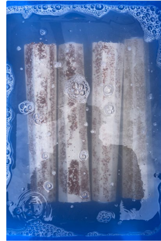
The four vases soaked in soapy water to dissolve excess glue, prior to final sanding.
