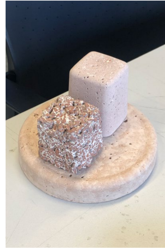
Using brick as a pigment and an aggregate. Radiant at first, the colour of the pigment rapidly faded.
