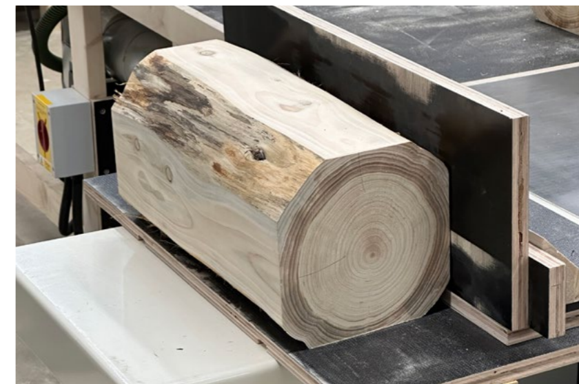
Four faces were cut along the lengths of the logs in an order which ensures perpendicularity.
