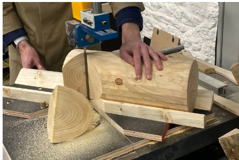
③ A final jig allowed two perpendicular cuts on both the plinth and gnomon; able to pivot 90° about the centreline of the blade without removal of the workpiece.
