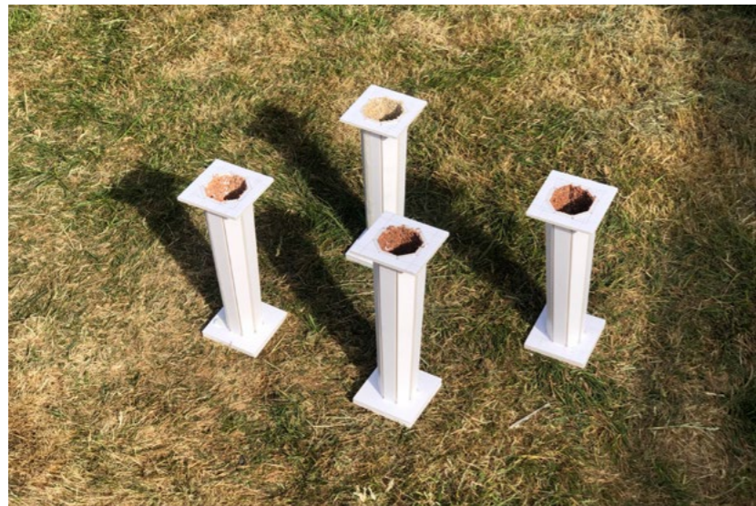
Four moulds—each lined with a different colour of brick—ready for concrete to be poured.
