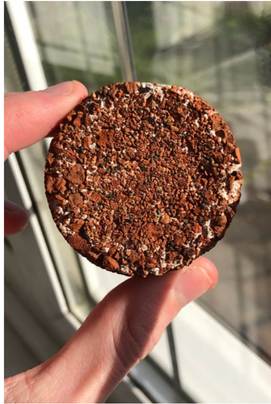
An experiment with Jesmonite, cast in a yoghurt pot coated in water soluble glue and sprinklings of disintegrated brick.
